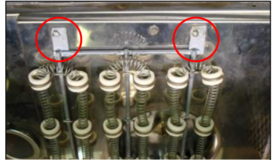
Figure 22. Remove Heater Panel by Removing Screw in Front Edge of Each Panel.
