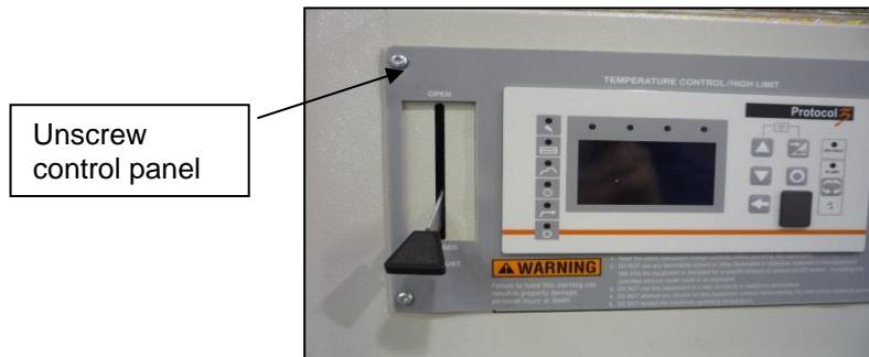
Figure 11. Control panel removal.
